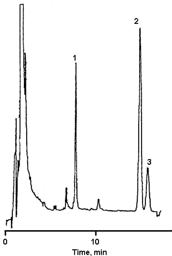
Fig. 3. SFE–LC of polymer additives (1000 \mu\text{g/g} each additive) from 20% cross linked PMMA prepared in-house, ground 2 \times , and sieved. See Table 1 for chromatographic conditions.
